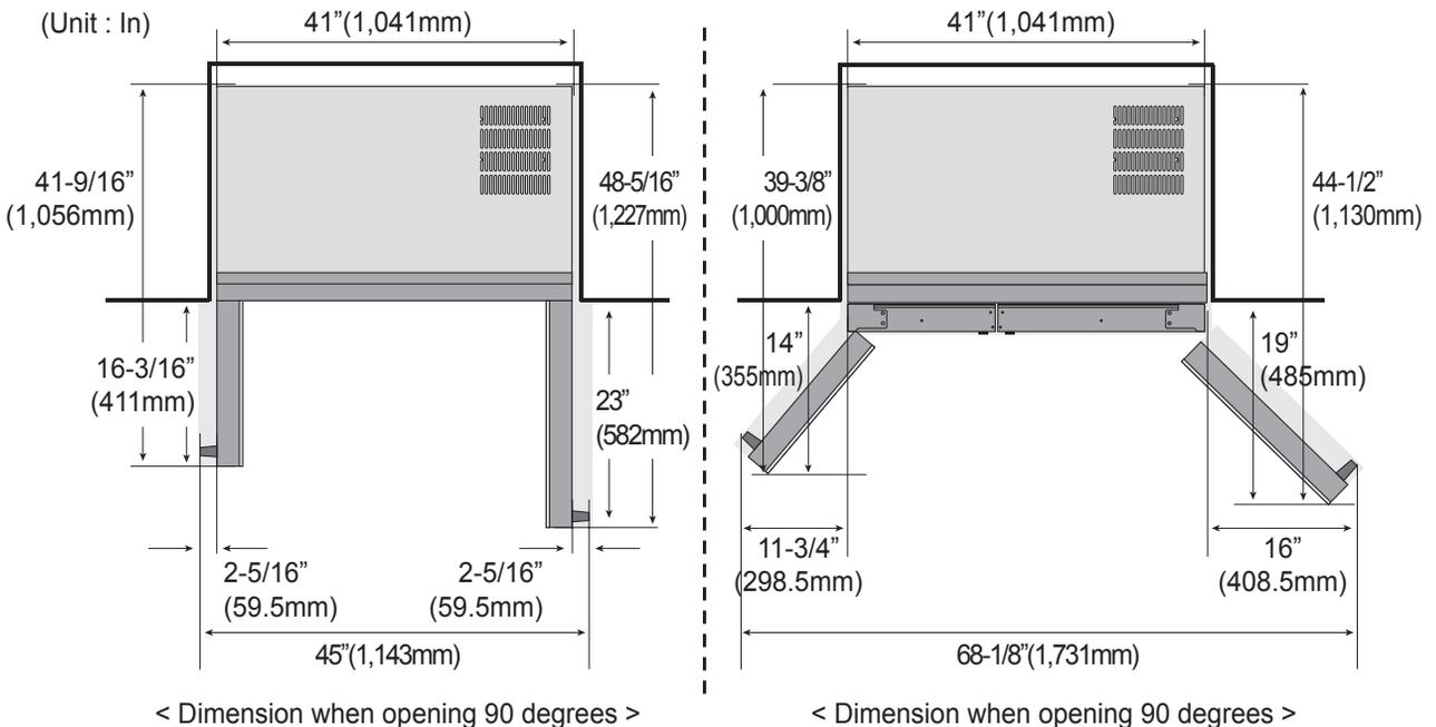
When installing the product on the wall near the corner, check the marked dimension to keep minimum distance to avoid the handle hitting the wall.
