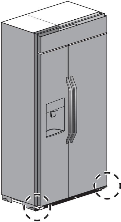
1) If the height of the refrigerator and freezer is different, turn the bottom door height adjustment bolt to adjust the height.
