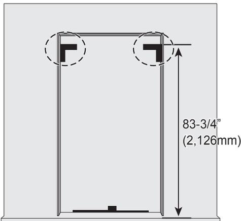
※ Because the built-in product is heavy on the top, the cabinet must be fixed firmly so that the product does not move when using it.
