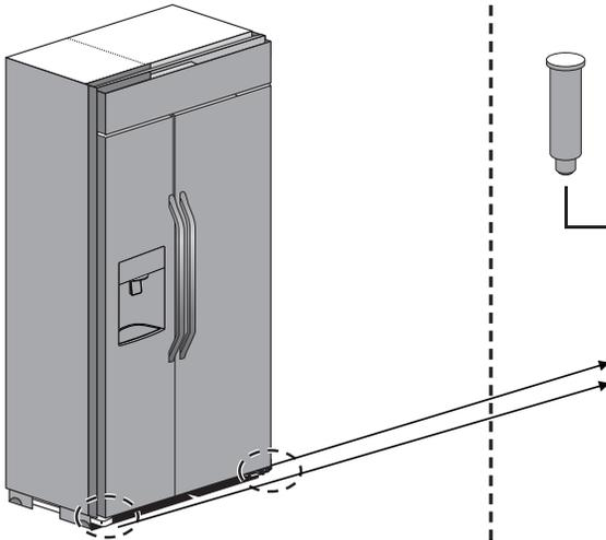
Push and install the device to keep the refrigerator door open and fixed, included in the accessory box, to the hole marked on the picture completely.
