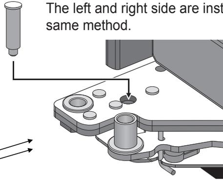
※ If the device to keep the refrigerator door open and fixed cannot be inserted, move the refrigerator door slowly in left and right direction to push it in.
